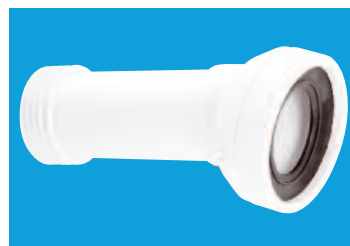
14° Angle Adjustable Length 97-107mm Inlet 3½"/90mm Outlet
