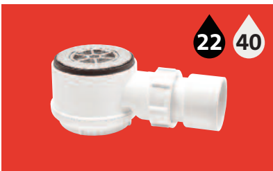
20mm Water Seal Trap with 1½" Solvent Weld Outlet Socket Overall height 65mm
