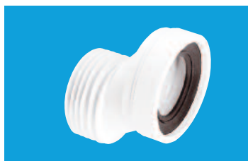
40mm Offset Adjustable Length 97-107mm Inlet 4"/110mm Outlet
